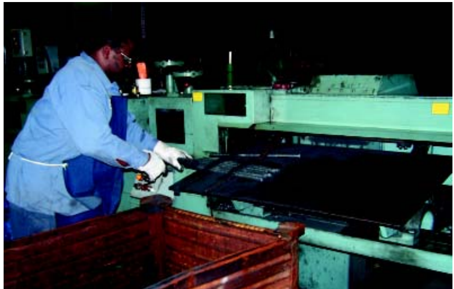
Coil stock is fed into the new shear (inset photo) as shear operator, Everett Bates, collects and stacks bars that have been cut.
